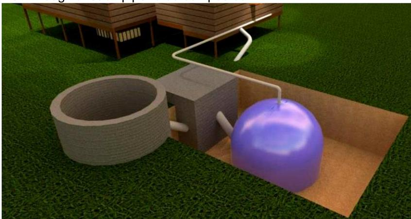
**Fig. 6** Illustration of making biogas processing equipment in Banjar tribe's traditional house
