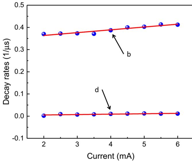
**Fig. 4.** The decay rates vs the discharge current. Solid lines are linearly fit to Eq. (2) and Eq. (3).
