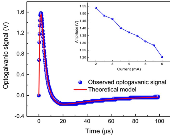
**Fig. 5.** Time-resolved optogalvanic signal of xenon at 473.54 nm corresponding to  $\Delta J = 1$ ,  $\Delta K = 0$  selection rules. The signal is recorded at 3 mA discharge current. The inset shows the decrease in the amplitude as a function of discharge current.
