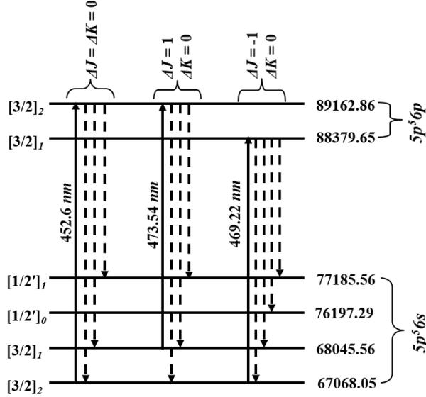
**Fig. 1.** Partial energy level diagram of xenon transitions.
