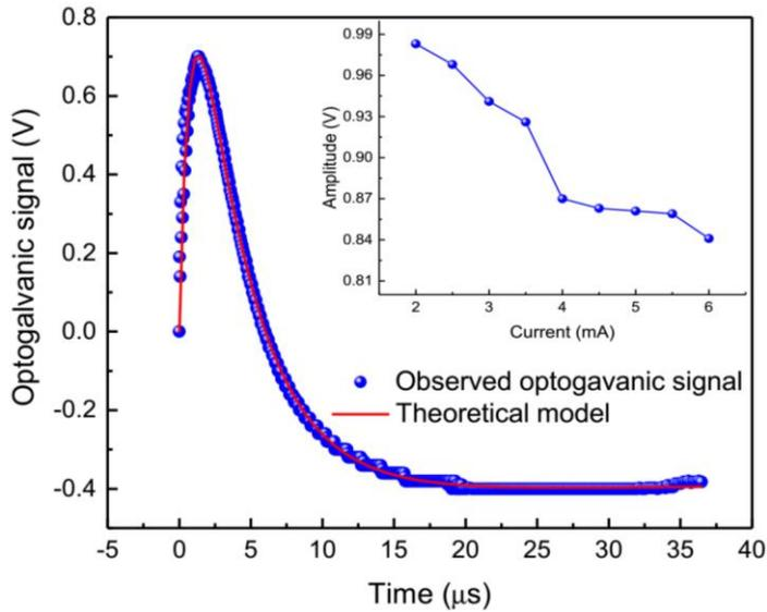
**Fig. 7.** Time-resolved optogalvanic signals of xenon at 452.6 nm corresponding to  $\Delta J = \Delta K = 0$  selection rules. The signal was rerecorded at 3 mA discharge current. The inset shows amplitude vs discharge current.
