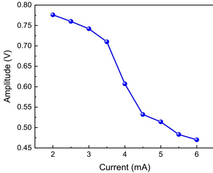
**Fig. 3.** The optogalvanic signal amplitude vs discharge current. The signal decreases with the increase of the discharge current.
