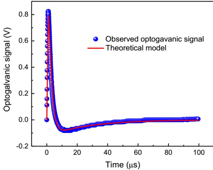
**Fig. 2.** Time-resolved optogalvanic signal of xenon at 469.22 nm and 2 mA discharge current following the  $\Delta J = -1, \Delta K = 0$  selection rules.
