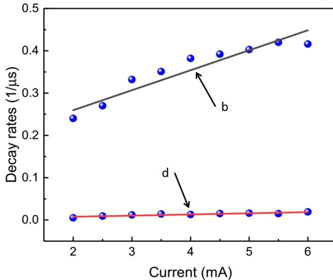
**Fig. 6.** The decay rates vs discharge current for xenon 473.54 nm. The solid lines are linearly fit to Eq. (2) and Eq. (3).
