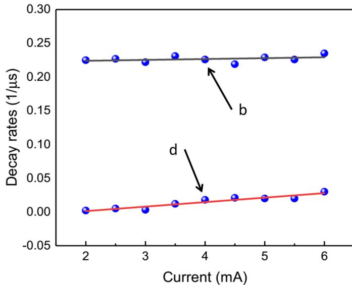
**Fig. 8.** The decay rates vs discharge current for xenon 452.6 nm. The solid lines are linearly fit to Eq. (2) and Eq. (3).
